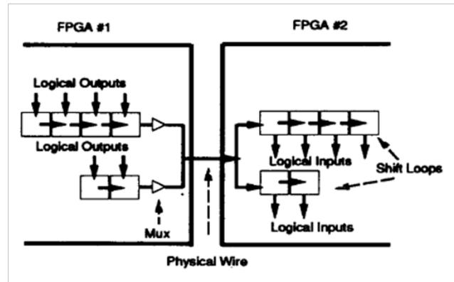
In the early 1990s, one of the major uses of FPGAs was ASIC emulation. The emulator system could include dozens or hundreds of FPGAs, but each FPGA might be only 10% occupied with logic. The low utilization was a result of the limited pins available for inter-FPGA communication and by the impracticality of re-partitioning and re-routing all those FPGAs for each modification of the ASIC design as it was debugged.
